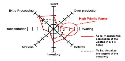
Figure 1: The Kiviat diagram and an example of high priority waste
